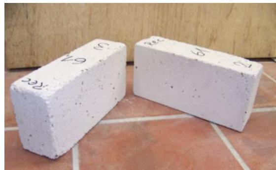
50 M.-% Beton-Recycling-Material (2/4 mm),
