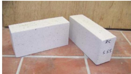
50 M.-% Beton-Recycling-Material (0/2 mm)
